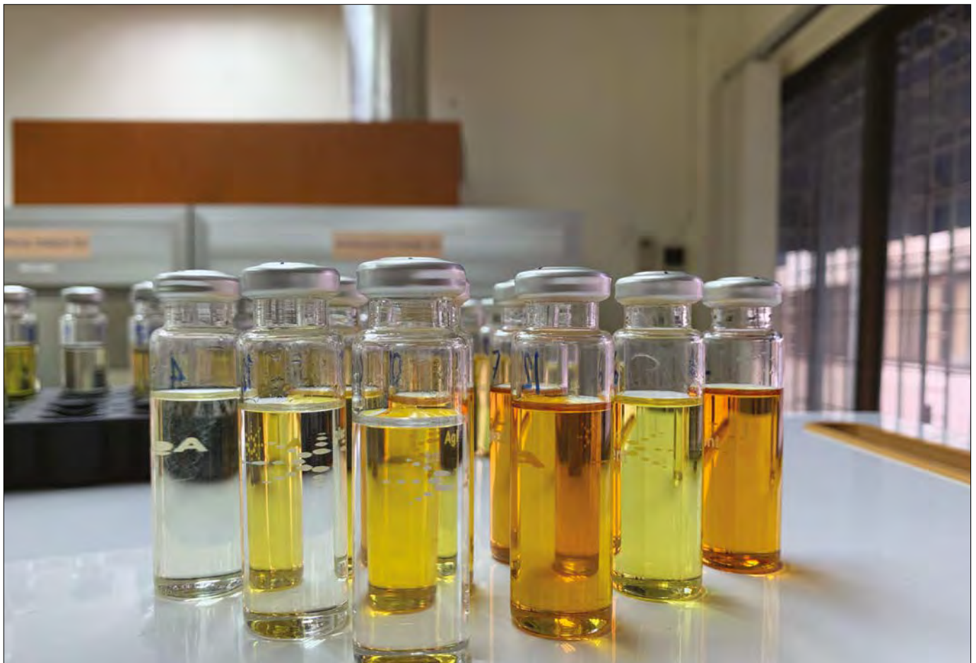
Figure 5. Dissolved Gas Analysis Test (DGA) for transformer oil
