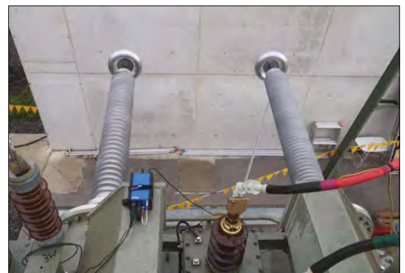
Figure 2. Setup for PD measurements on phases 1U and 1V
